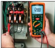
True RMS multimeter gives accurate readings of distorted waveforms
