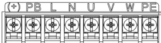
Fig 3.4 1PH terminals of main circuit
