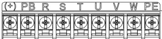
Fig 3.5 3PH terminals of main circuit
