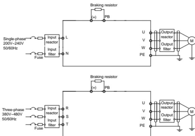
Fig 3.3 Connection diagram of main circuit
