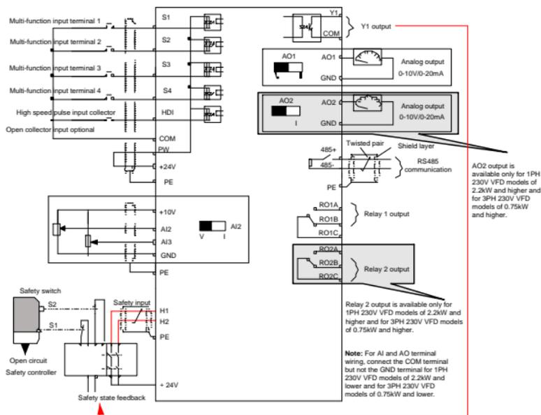
Fig 3.7 Wiring of control circuit of G200UL-02versions
