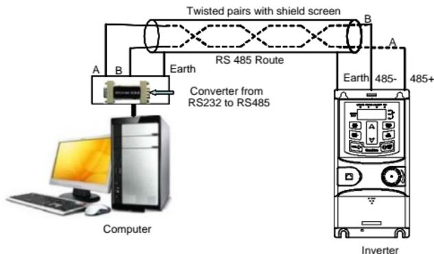
Fig 7.1 RS485 physical connection in single application
