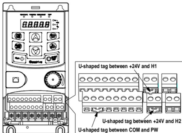
Fig 3.9.2 U-shaped contact tag of G200UL-02 versions
