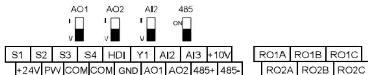
Fig 3.8 Terminals of control circuit
