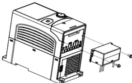
The installation procedures for C3 filter are as below:
