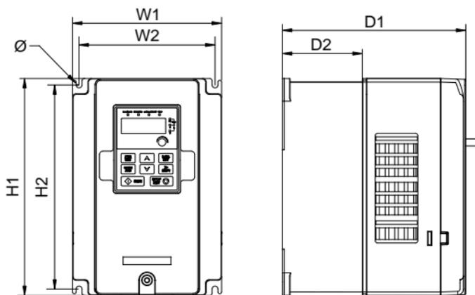
Wall mounting of 3PH 400V 4–11kW and 3PH 230V 1.5–2.2kW VFDs
