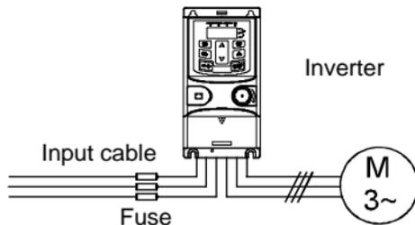
Fig 3.12 Fuse configuration
