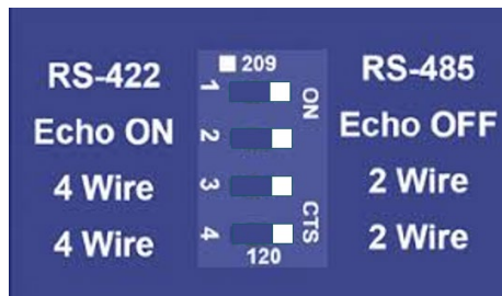
Figure 13: Dip Switch settings
