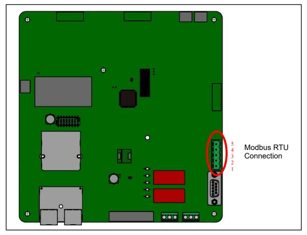
**Figure 11: PQconnect Modbus RTU Connection**
