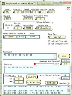
Select "0" in the field "Values to Write" to close the contactor or "1" to open the contactor.
