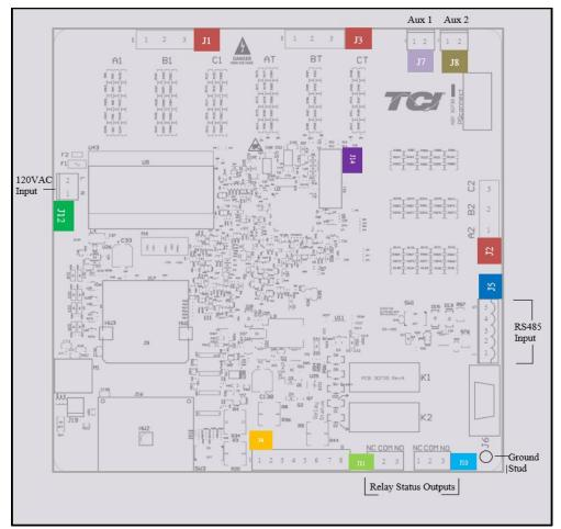
Figure 10: PQconnect Connections
