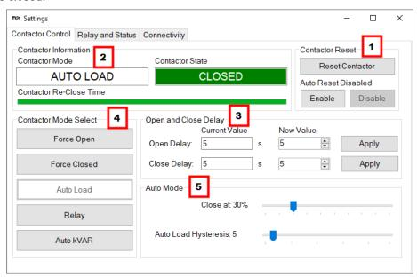
**Figure 5: Contactor Control Settings Menu**
