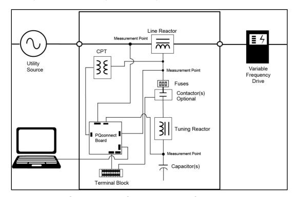
Figure 3: HGL Filter with PQconnect Typical Connection Diagram
