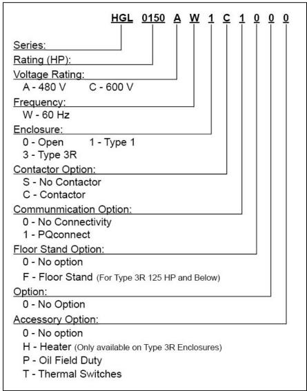
Figure 1: HGL Part Number Encoding
