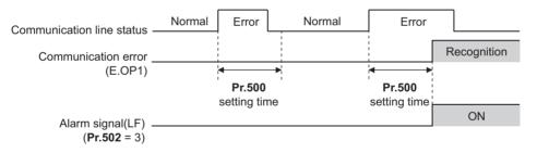
When a communication line error occurs and lasts longer than the time set in **Pr.500**, it is recognized as a communication error. If the communication returns to normal within the time, it is not recognized as a communication error, and the operation continues.
