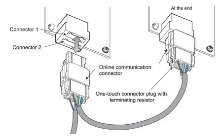
Use the following online communication connector and one-touch connector plug with terminating resistor.
