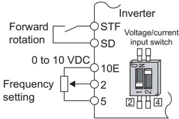
Connection diagram using terminal 2 (0 to 10 VDC)
