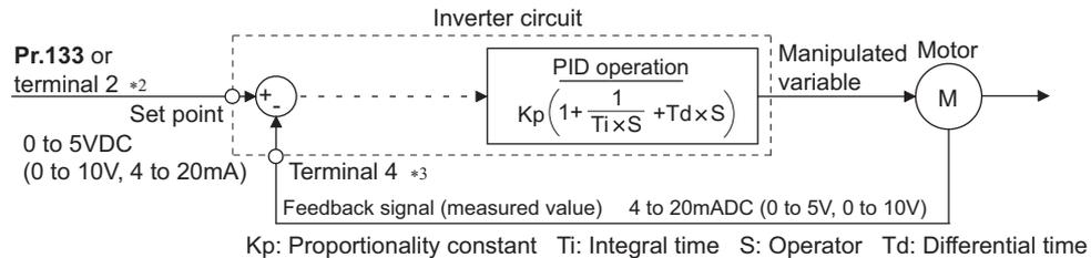
\*2 Note that the input of terminal 1 is added to the set point of terminal 2 as a set point.
