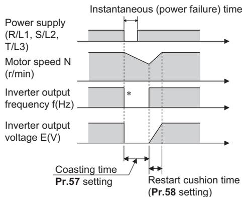
\* The output shut off timing differs according to the load condition.
