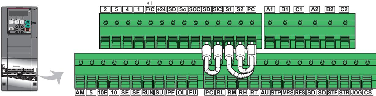
\*1 This terminal operates as the terminal FM for the FM type, and as the terminal CA for the CA type.
