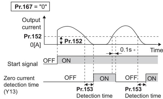
\* When the output is restored to the Pr.152 level, the Y13 signal is turned OFF after 0.1 s.
