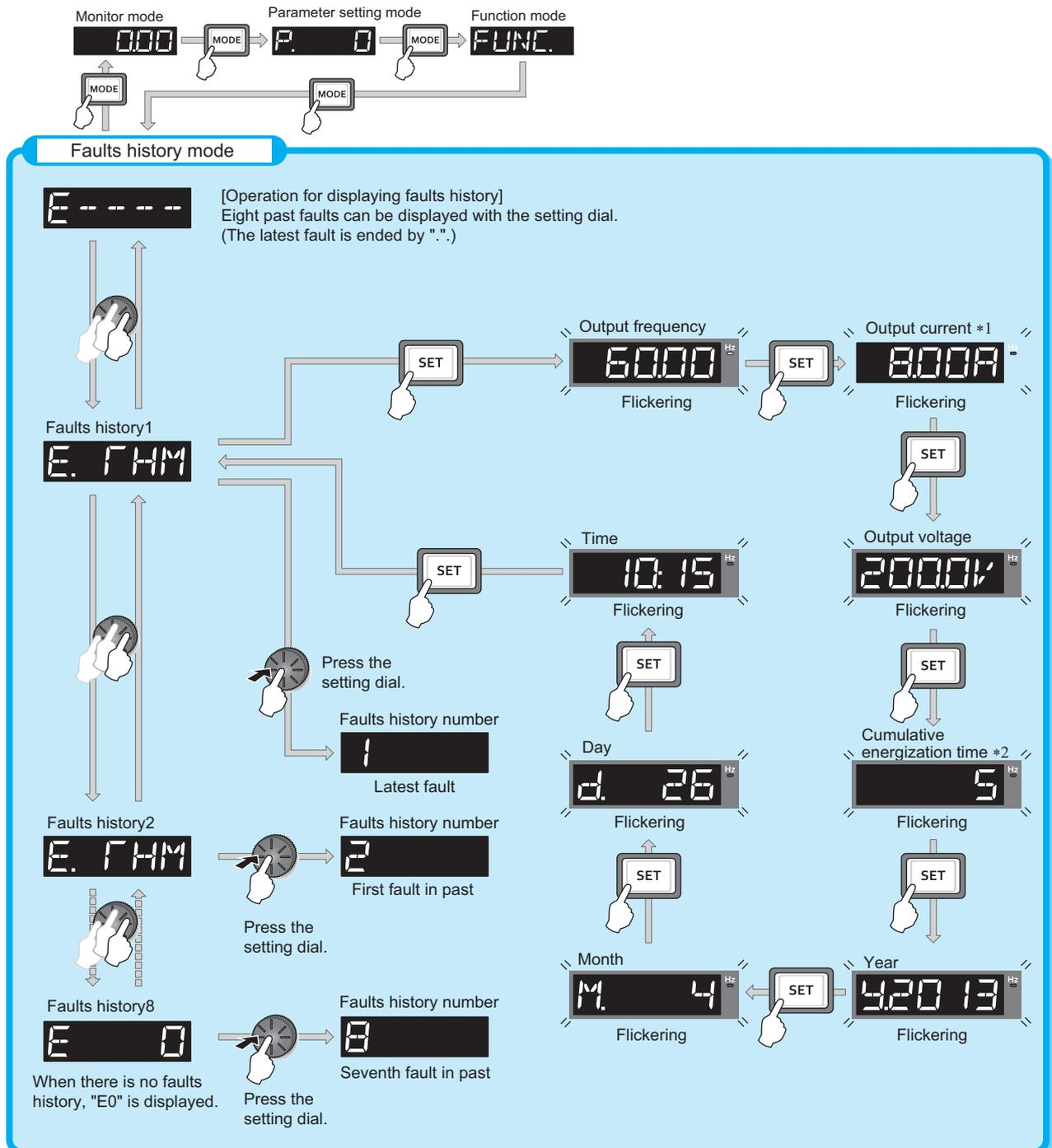
\*1 When an overcurrent trip occurs by an instantaneous overcurrent, the monitored current value saved in the faults history may be lower than the actual current that has flowed.
