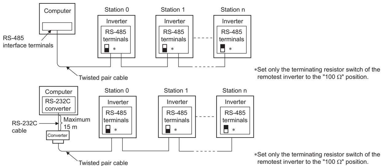
\*Set only the terminating resistor switch of the remotest inverter to the "100 Ω" position.
