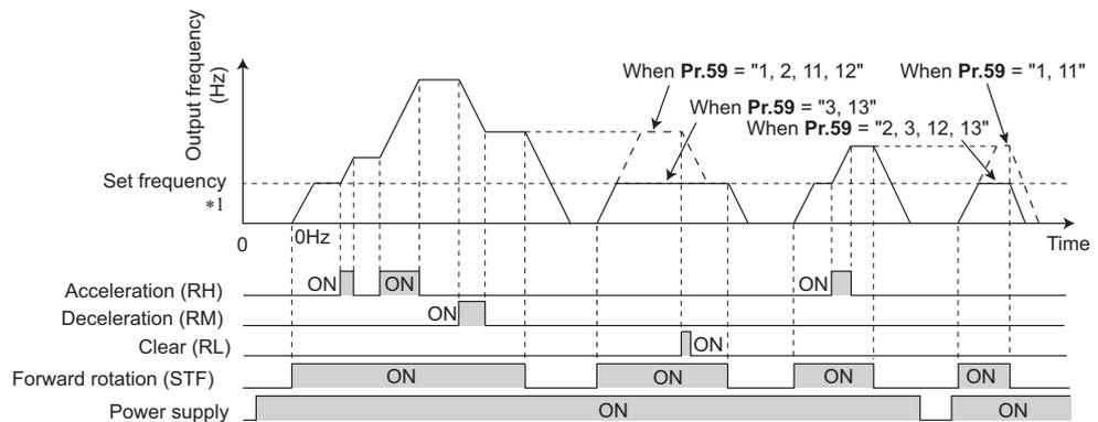
\*1 External operation frequency (other than multi-speed) or PU running frequency
