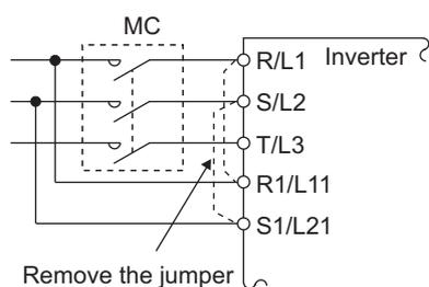
When a fault occurs, opening of the electromagnetic contactor (MC) on the inverter power supply side results in power loss in the control circuit, disabling the fault output signal retention. Terminals R1/L11 and S1/L21 are provided to hold a fault signal. In this case, connect the power supply terminals R1/L11 and S1/L21 of the control circuit to the input side of the MC.
