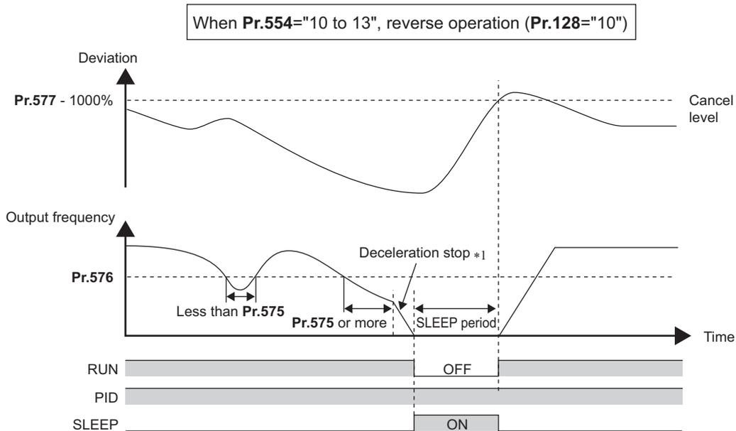
\*1 When the PID output shutoff release level is reached during a deceleration stop, output shutoff is released, operation is re-accelerated and PID control is continued. During deceleration **Pr.576 Output interruption detection level** is invalid.
