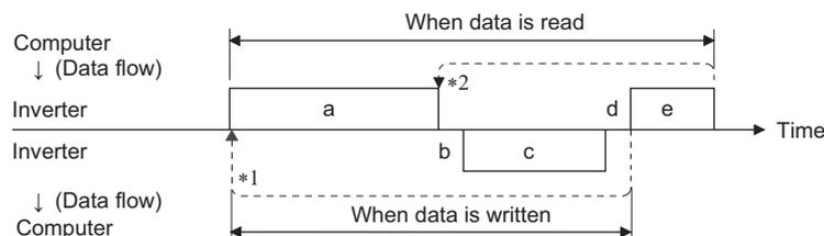
\*1 If a data error is detected and a retry must be made, perform retry operation with the user program. The inverter trips if the number of consecutive retries exceeds the parameter setting.
