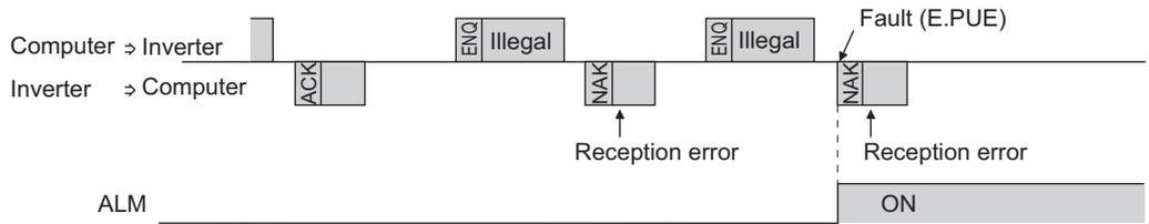
Example: PU connector communication, Pr. 121 = "9999"
