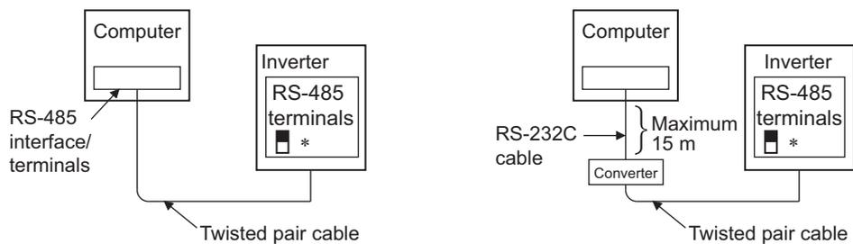
\*Set the terminating resistor switch to the "100 Ω" position.
