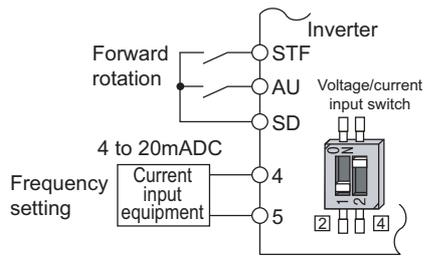
Connection diagram using terminal 4 (4 to 20mADC)
