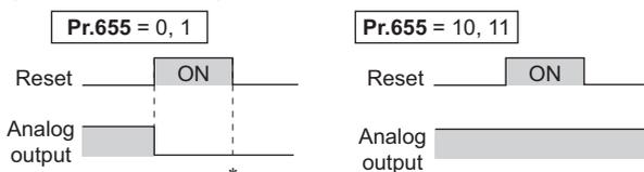
\* When **Pr.655** = "1", the signal condition saved in EEPROM (condition of the last power OFF) is applied.
