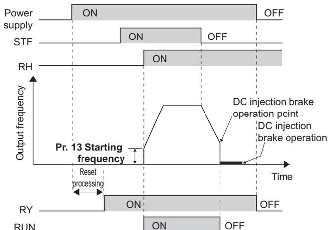
(c) Checking the inverter operating status by the start signal input to the inverter and inverter running signal
