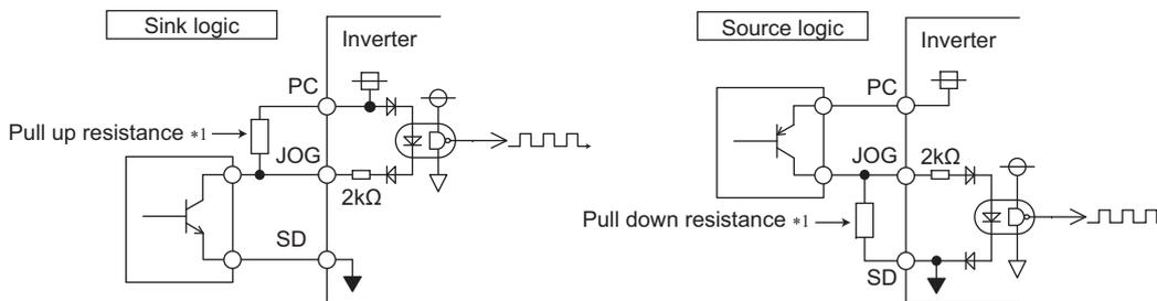
\*1 When the wiring length is long with open collector outputs, the influence of stray capacitance causes the pulse to flatten out and prevents the input pulse from being recognized.
