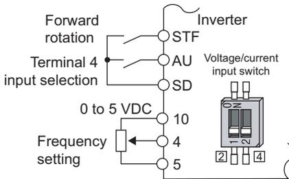
Connection diagram using terminal 4 (0 to 5 VDC)
