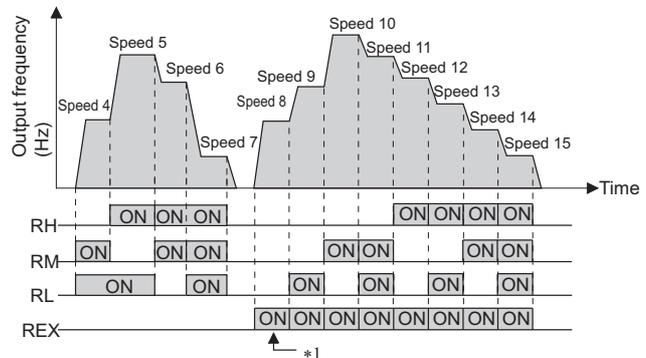
\*1 When RH, RM and RL is set to OFF and REX is set to ON when "9999" is set to **Pr.232 Multi-speed setting (speed 8)**, the inverter runs by the frequency set to **Pr.6**.
