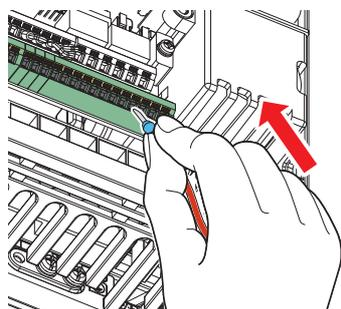
When using a single wire or stranded wires without a blade terminal, push the open/close button all the way down with a flathead screwdriver, and insert the wire.
