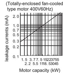
For "Δ" connection, the amount of leakage current is approx. 1/3 of the above value.
