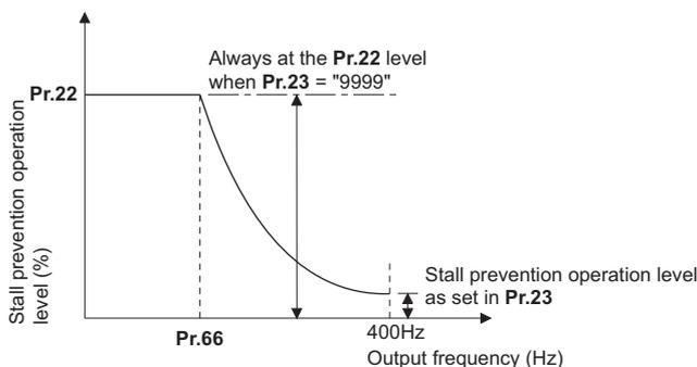
Setting example (Pr.22 = 150%, Pr.23 = 100%, Pr.66 = 60Hz)
