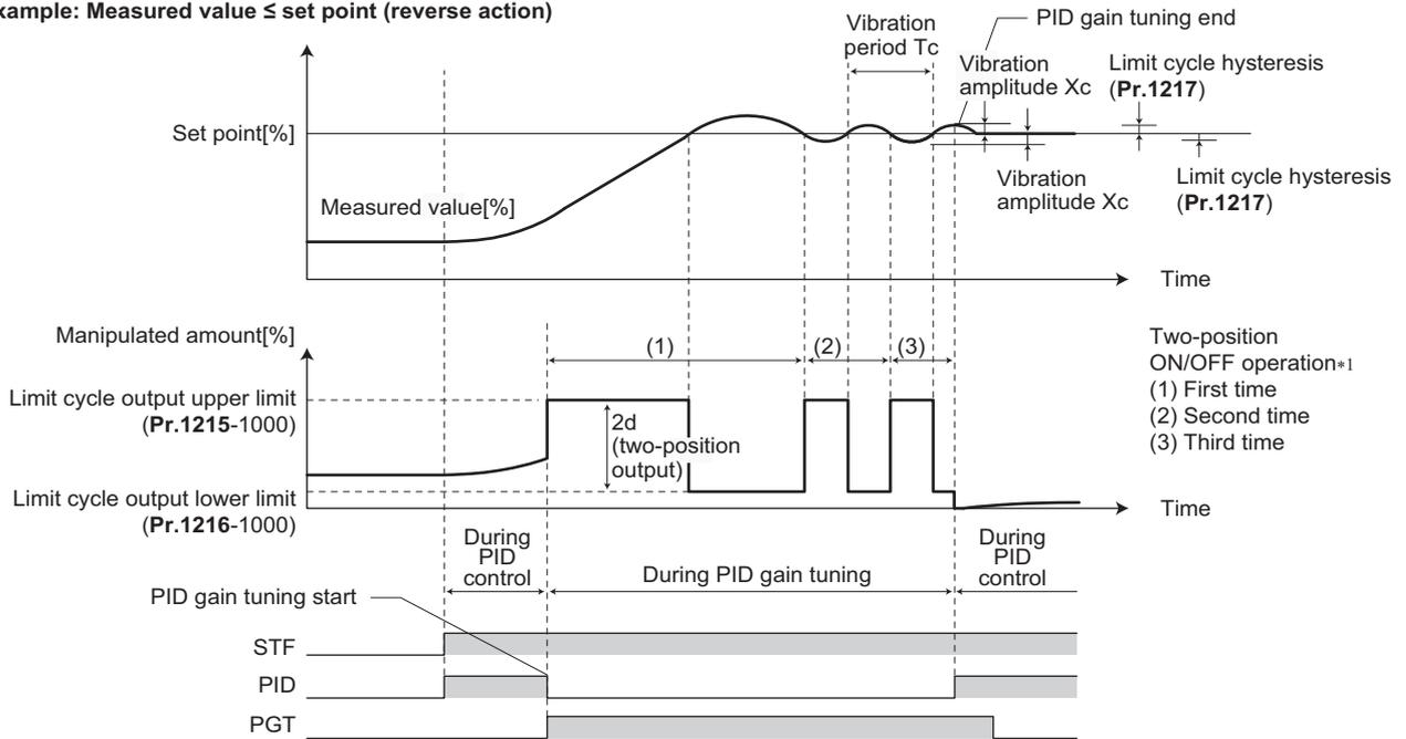
\*1 Details of the two-position ON/OFF operation
