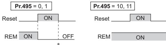
\* When **Pr.495 = "1"**, the signal condition saved in EEPROM (condition of the last power OFF) is applied.
