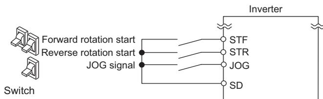
**Operation example** Operate at 5 Hz.
