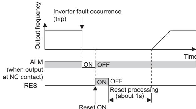
(b) Checking the inverter operating status by the inverter operation ready completion signal
