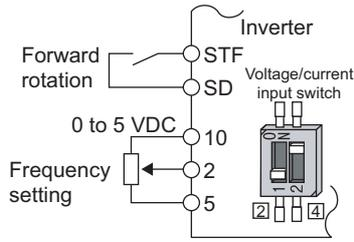
Connection diagram using terminal 2 (0 to 5 VDC)
