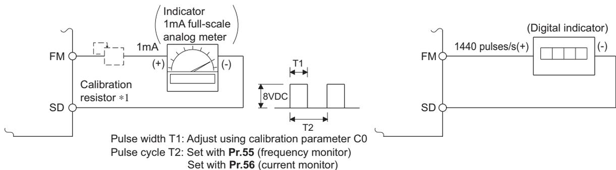
\*1 Not needed when the operation panel or the parameter unit is used for calibration.
