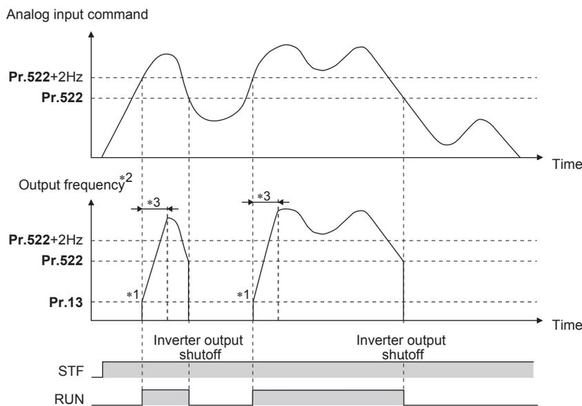
\*1 At a stop condition, the motor is accelerated at the **Pr.13 Starting frequency** (0.01 Hz under PM motor control).
