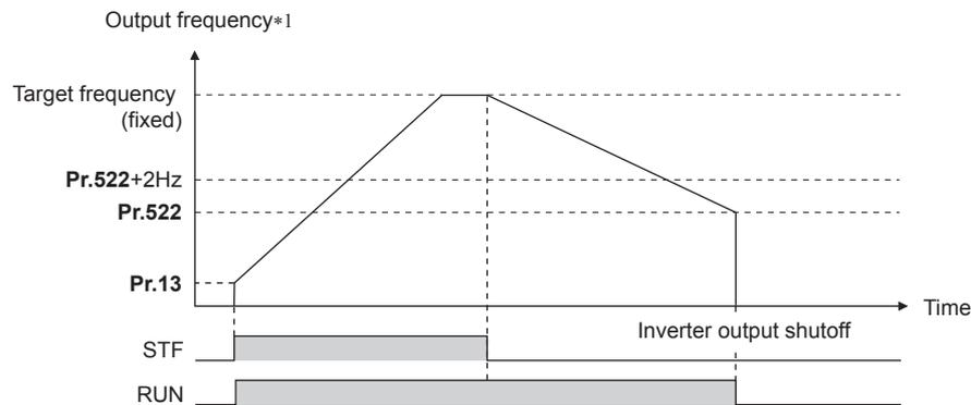
\*1 The output frequency before the slip compensation is compared with the **Pr.522** setting.
