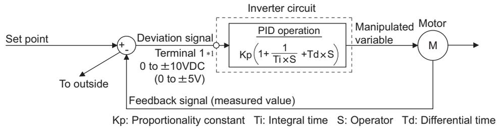
\*1 Set "0" to Pr.868 Terminal 1 function assignment. When Pr.868 ≠ "0", PID control is invalid.
