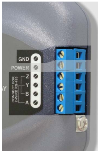
Figure 3: Terminal Block RS-485 Connections
