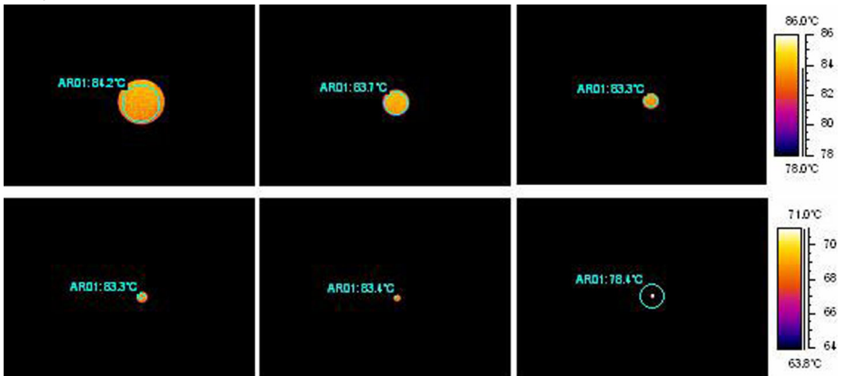
Figure 17.20 Temperature readings from a blackbody at +85°C (+185°F) at increasing distances (24° lens)
