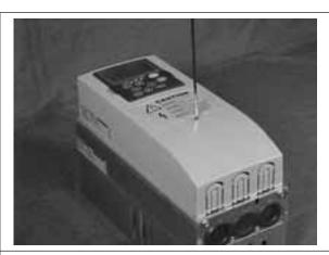
2. Remove the bottom cover by rotating the cover towards you on the base hinges, then lifting the cover away from the base.
