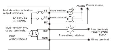
Multi-function Terminals Wiring Example
