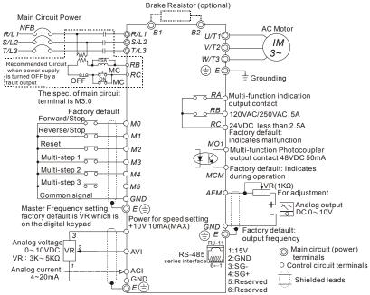
NOTE: Do not plug a Modem or telephone line to the RS-485 communication port, permanent damage may result. Terminal 1& 2 are the power sources for the optional copy keypad and should not be used while using RS-485 communication.
