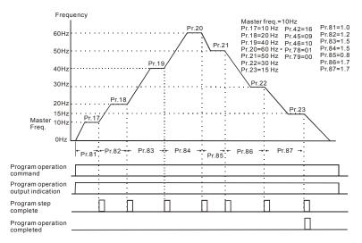
Note: The above diagram shows one complete PLC cycle. To restart the cycle, turn the PLC Program input off and then back on.
