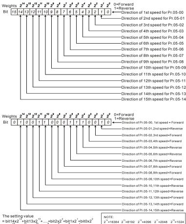
= bit4x2<sup>-1</sup> +bit3x2<sup>-1</sup> +...+bit2x2<sup>2</sup>+bit1x2<sup>1</sup>+bit0x2<sup>0</sup> = 1x2<sup>-1</sup> +1x2<sup>-1</sup> +1x2<sup>-1</sup> +1x2<sup>2</sup> +1x2<sup>2</sup> +1x2<sup>1</sup> +1x2<sup>1</sup> = 13384+2048+1024+64+32+16+2 =19570 Setting 05-16
