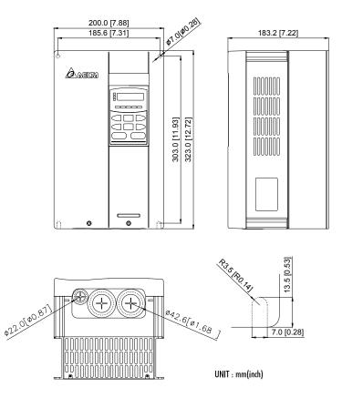
Frame D: VFD150B23A/43A/53A, VFD185B23A/43A/53A, VFD220B23A/43A/53A
