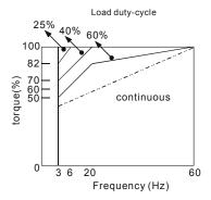
If 100% continuous torque is required at low speed, it may be necessary to use a special inverter duty motor.
