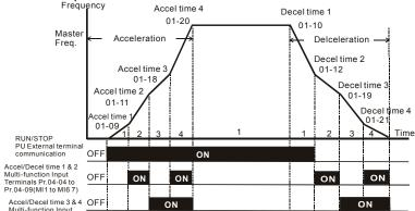
Multi-function Input Terminals Pr.04-04 to Pr.04-09(MI1 to MI6 8)
