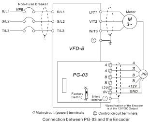
2. Connect Externally with the Encoder of 12V Power Supply and Output Signals to
