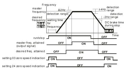
output timing chart of multiple function terminals when setting to frequency attained or zero speed indication
