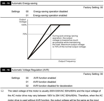
voltage. When the motor runs at voltages exceeding the rated voltage with 12% - 20%, its lifetime will be shorter and it can be damaged due to higher temperature, failing insulation and unstable torque output.
