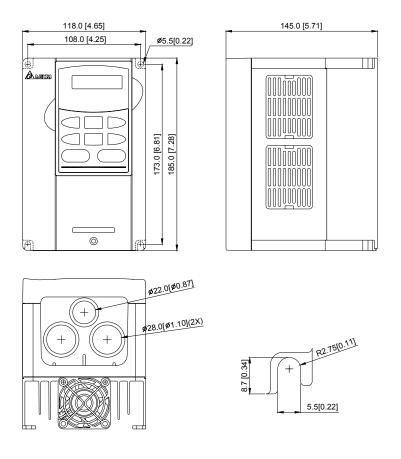
Frame B: VFD022B21A, VFD037B23A/43A/53A
