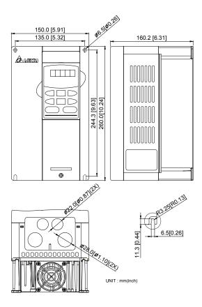
Frame C: VFD055B23A/43A/53A, VFD075B23A/43A/53A, VFD110B23A/43A/53A
