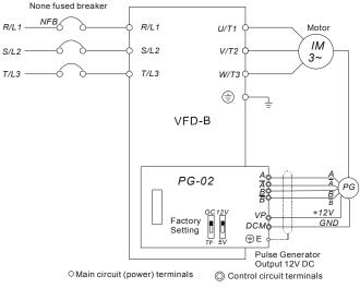
PG-02 and Pulse Generator Connections
