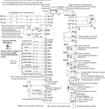
Figure 4 Wiring for SINK mode and SOURCE mode
