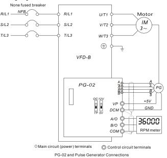
3. When Pulse Generator (Encoder) is Open Collector type, please refer to following wiring.
