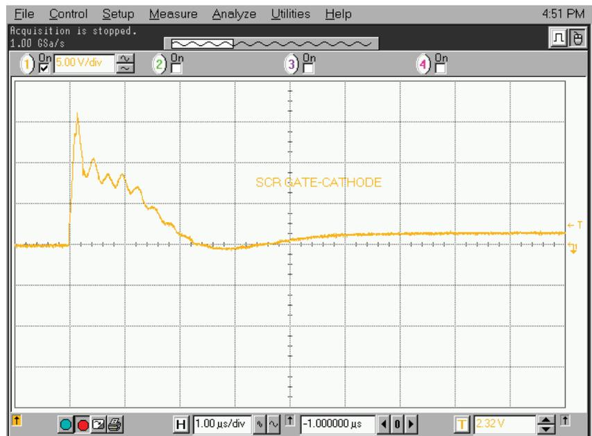
Figure 263 - V Sense Trigger to SCR gating pulse
