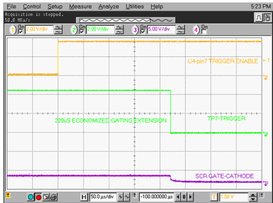
Figure 97 - Expansion of V Sense Trigger to SCR Gating Pulse
