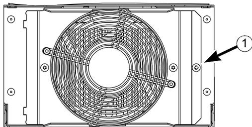
2. Open the swing-out frame and disconnect the cable.
