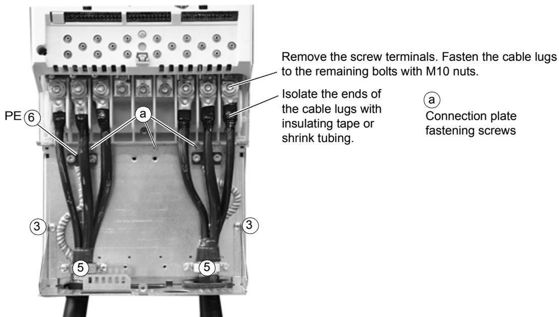
Frame size R6: Cable terminal installation [95 to 240 mm<sup>2</sup> (3/0 to 500 MCM) cables]
