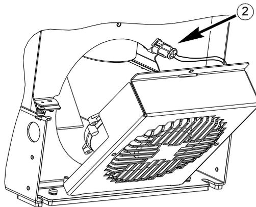
3. Take off the casing and replace the fan onto the casing's pins.
