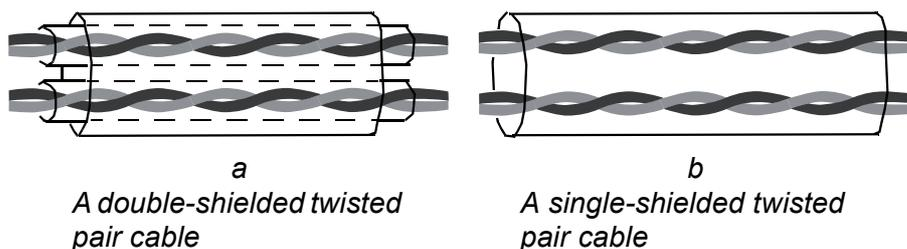
Run analogue and digital signals in separate, shielded cables.
