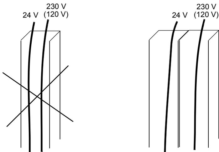
Not allowed unless the 24 V cable is insulated for 230 V (120 V) or insulated with an insulation sleeving for 230 V (120 V).
