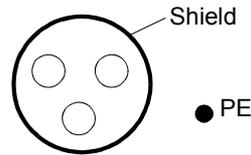
A four-conductor system: three phase conductors and a protective conductor
