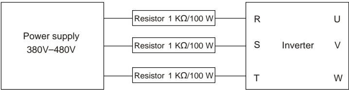
Figure 8-2 Charging circuit example of driving devices of 460 V
