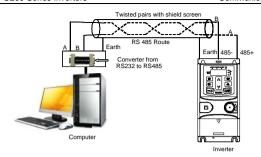
Fig 7.1 RS485 physical connection in single application
