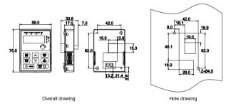
The external keypad can be mounted on the installation bracket and the bracket is optional.
