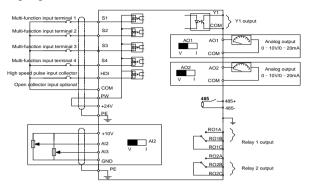
Fig 3.6 Wiring of control circuit of G200UL-01 versions
